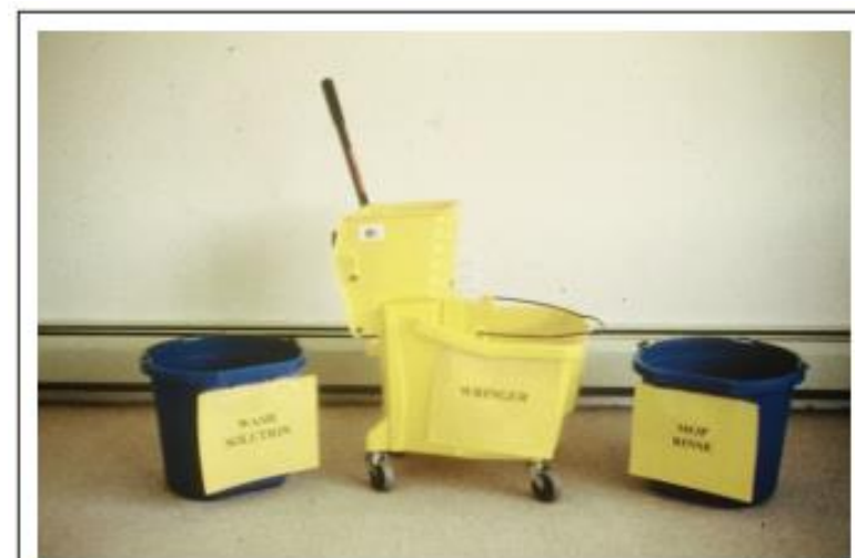
FIGURE 14.4 Three-bucket cleaning system.
